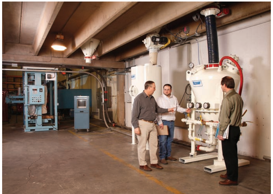
Test lab technicians talk with a customer about a dense-phase pressure conveyor's operating principle before conducting a test with a highly abrasive material.
